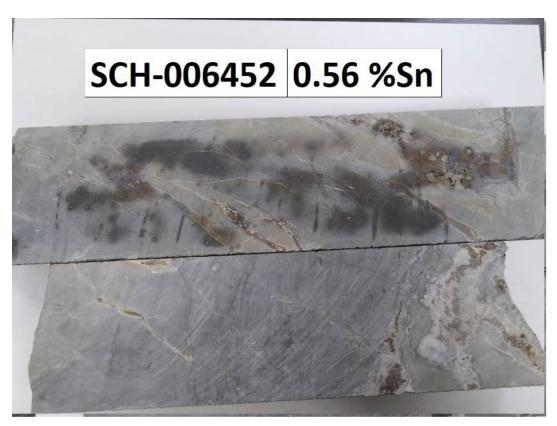
Figure 5: A 0.5m long section of Dowa core with alteration but no obvious sulfide and returned 0.56% tin and 0.34% zinc from WHG assay testing.
