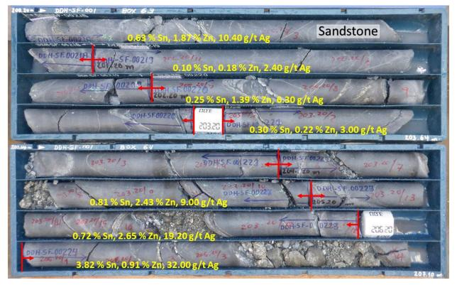
Figure 2. Polymetallic mineralization in core hole DDH-SF-001, from 200.20 m to 207.10 m.
